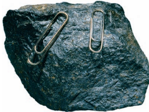
FIGURE 1.19 Lodestone, a variety of magnetite, is a weak magnet and will attract iron objects.
