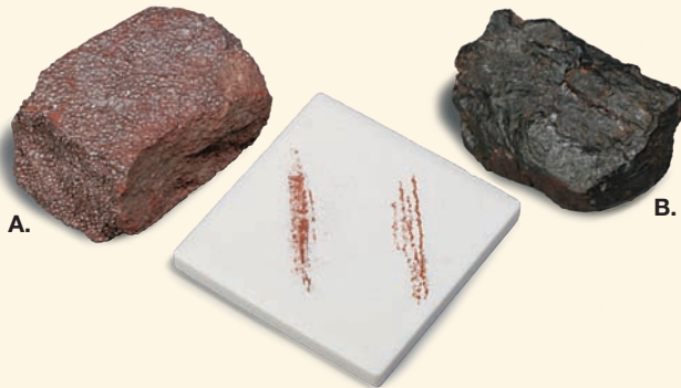
FIGURE 1.8 Hematite, an ore of iron, is found in both nonmetallic and metallic forms.
