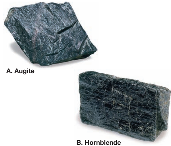
FIGURE 1.30 These dark-colored silicate minerals are common constituents of igneous rocks: A. Augite and B. Hornblende. (Photos by Dennis Tasa)
